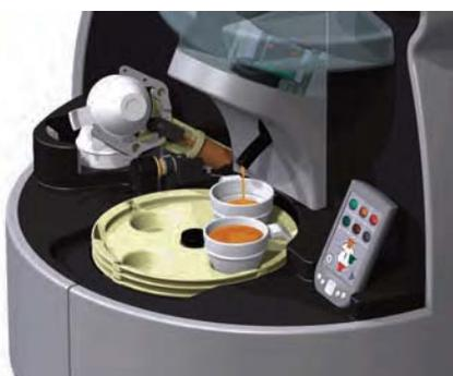
Fig. 2. The self-contained coffee machine permits automatic just-in-time positioning of cups on the tray. The cup tower constantly controls the position of the next cup and the number of remaining cups. After the prehensor places the cup on the tray, the latter turns to put the cup under the brewing head. In parallel, the capsule dispenser releases the correct blend. The brewing can start and the user can enjoy NESPRESSO's superior quality ground coffee.
